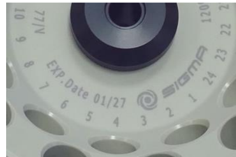
Fig. 2: Different service life – engraving on the bucket/rotor
